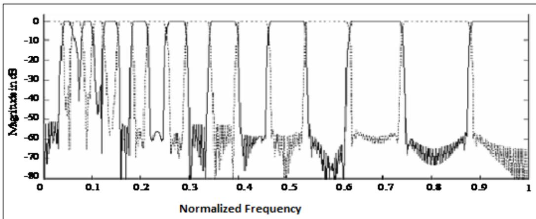
Fig. 1: Magnitude Response of Comb Filter.
