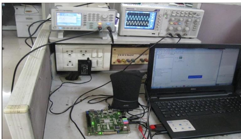
**Fig. 5: Experimental Setup for Comb Filter Implementation.**
