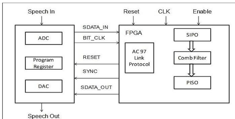
**Fig. 4: FPGA Implementation Schematic.**
