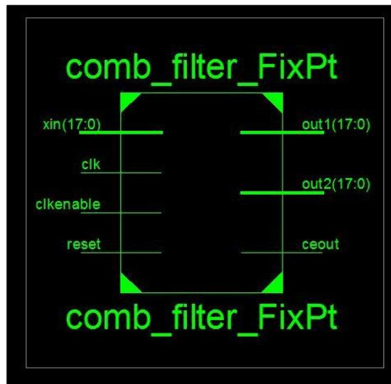
Fig. 7: RTL Schematic for Critical Band Filter.
