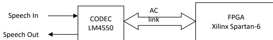
**Fig. 3:** Flow of Unprocessed and Processed Signal using FPGA.
